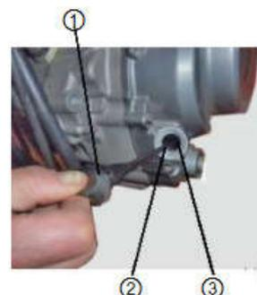
Insert the oil gauge into the lubricating oil (cannot be rotated) and take out the view.
